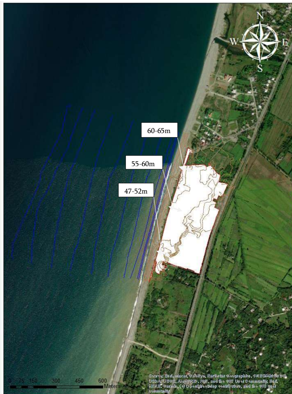
Fig. 1. The results of the topographic and bathymetric survey are mapped onto an aerial photograph using the Arc Gis tool, adding shore widths.
