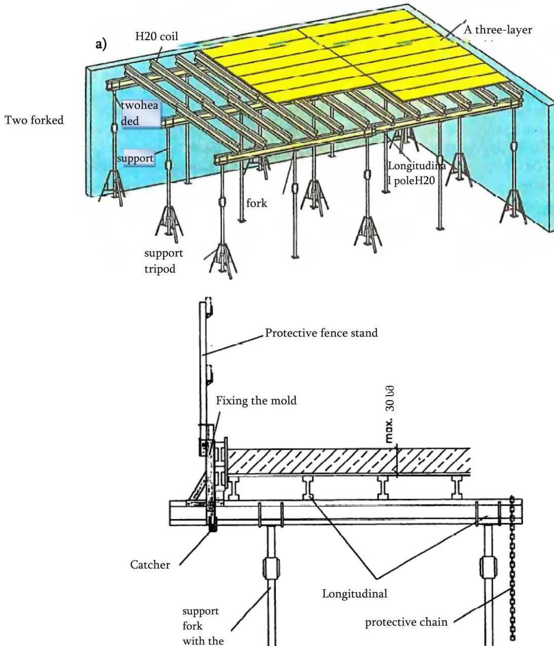
fig. 8. "Noes" roofing mold with H20 coils:
