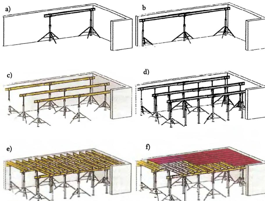
Fig. 2. „PASCHAL DEK“ Mold installation sequence: A Operation No. № 1; b – № 2; c – № 3; d – № 4; e – № 5; f – № 6
