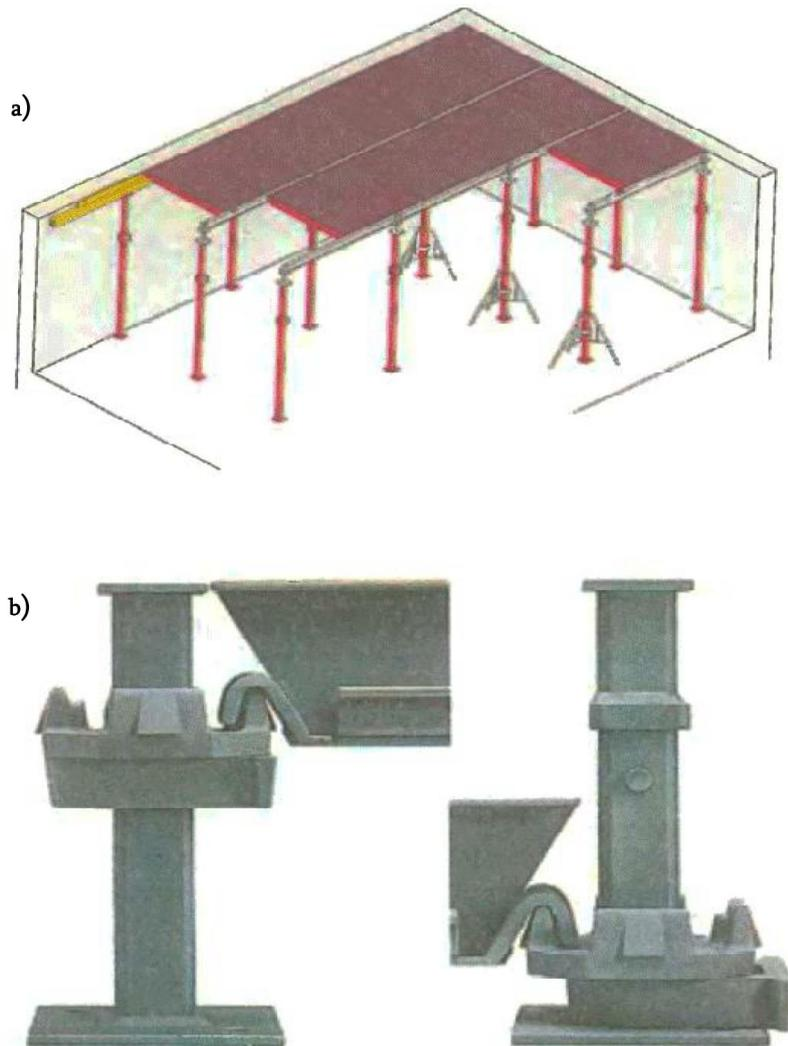
fig. 7. "Noes" roofing mold with falling heads: A - ceiling mold with falling heads; b - longitudinal Anvil with a falling head
