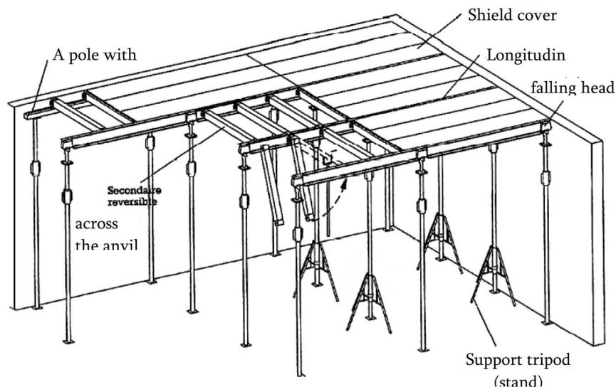
fig. 6. "Noes" roofing mold, expandable With telescopic spools and "swivel heads"
