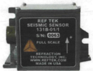
figs. 1. Accelerometer RefTek 131 V-01/1
