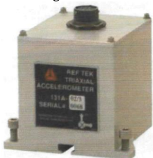
figs. 2. Accelerometer RefTek 131V-01/1 Seismic receiver six-channel RefTek 130-01
