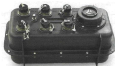
figs. 3. Six-channel recorder Reftek 130-01
