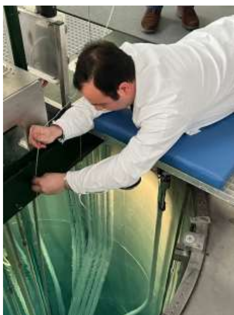
Figure 7. Inserting sample holders into the reactor core
