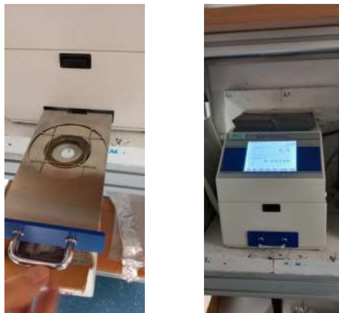
Figure 9. Measuring activity of irradiated foils using 4\pi\beta counter
