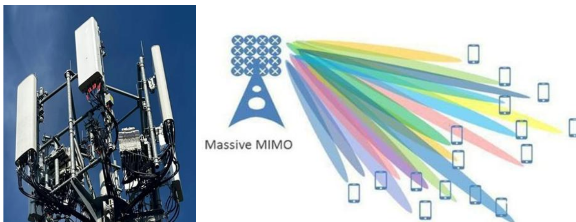
Figure 3. Massive MIMO antenna
