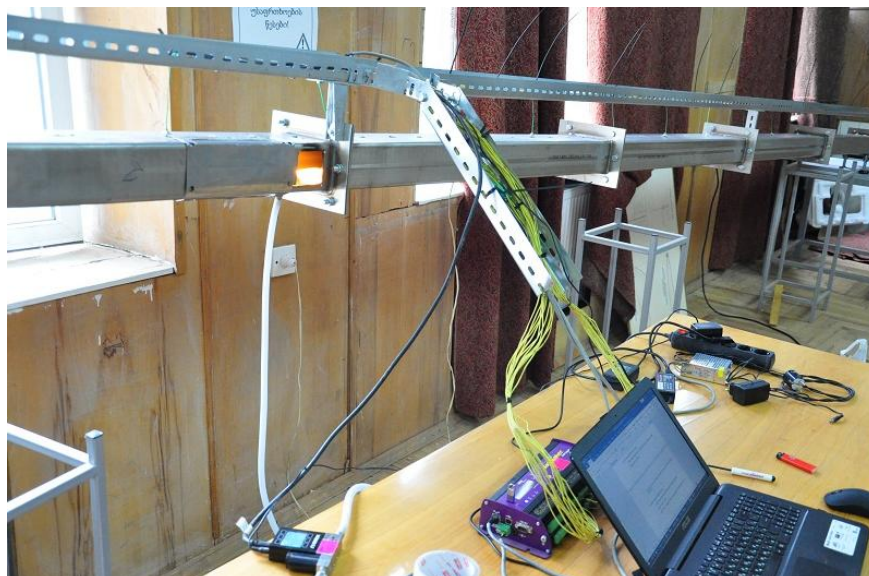
Fig. 3. Tunnel model with thermocouples and measuring instruments.
