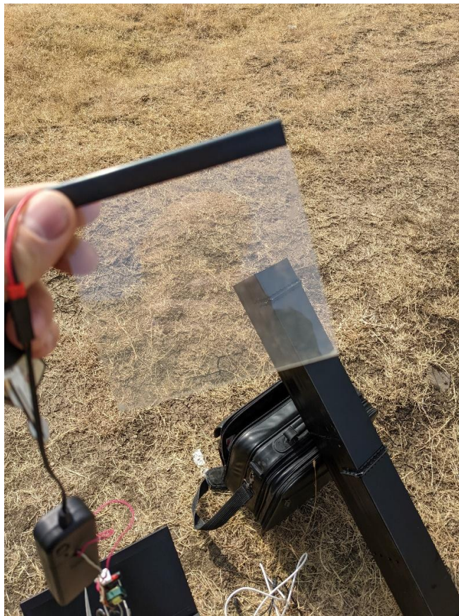
PDLC film when turned off (blurred)
