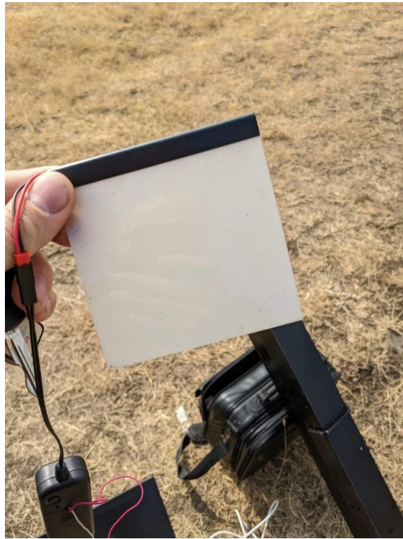
PDLC film when turned off (blurred)
