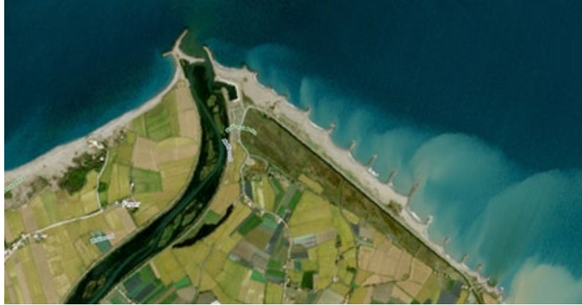
Figure 14. Protection of the banks from erosion east of the mouth of the Kizilirmak River with special spurs created in 1999-2010 (Sentinel-2)
