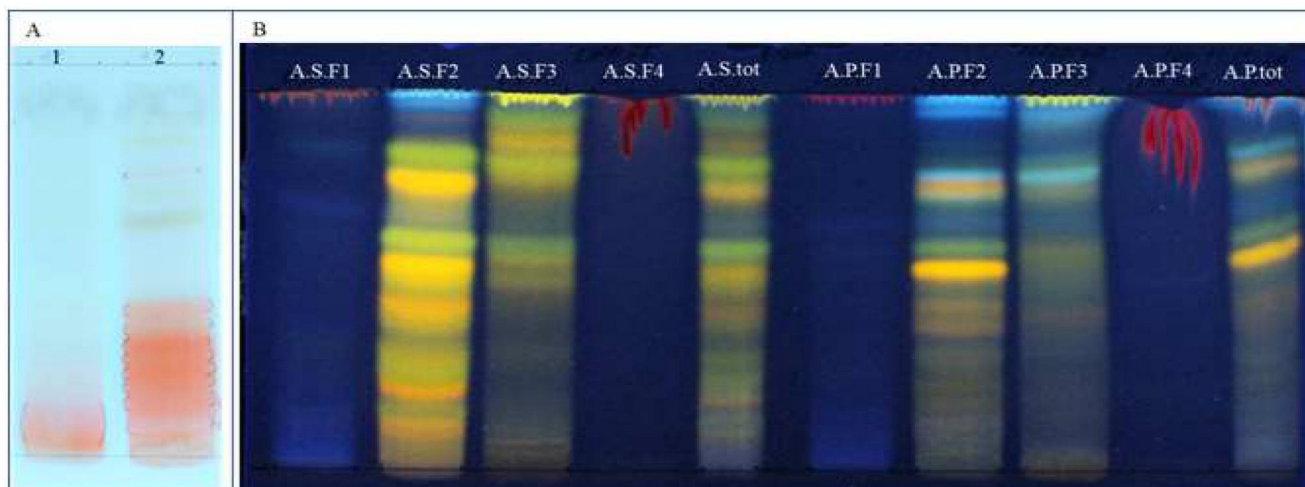
Figure 2. A-TLC of furostanolic saponins: 1-Crude extract of A. ponticum ; 2-Crude extract of A. Saxatile ; B-TLC of flavonoids under 366 nm wavelength
